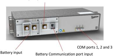
The Solar Inverter Interface SII includes an advanced communications interface that translates the standard ModBus used in Polarium batteries into various communication protocols. The SII comes with CAN, TCP/IP and can be fitted with customized protocols. Additionally the SII unit will ensure a smooth start-up sequence and limit the inrush current in the system
